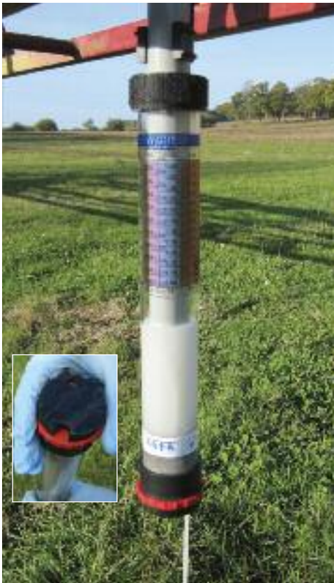
FlowCheck showing easily readable flow chart
