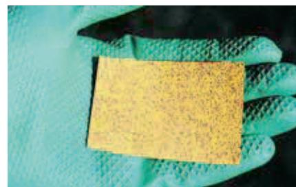
The special coating of hydro sensitive and oleo sensitive papers will enable you to evaluate spray coverage and the density of droplets. You can then check the spraying quality of your nozzles.
